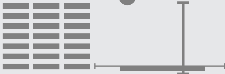
A conventional Storage and retrieval System with long buffer zones with lost space.
