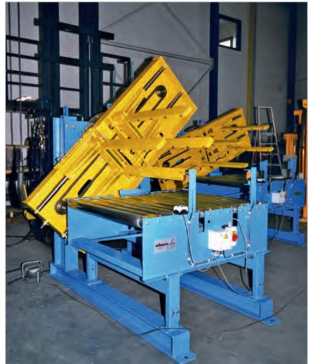
Turning unit to deburr castings with industrial robot
