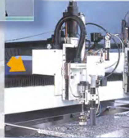
Franke linear table in a laser cutting plant. The linear table moves the machining head over the work piece quickly and precisely. The positioning accuracy is about 0.01 mm.
