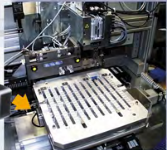
Franke linear tables in a pin-mounting machine. The metal cover of the tables protect the guide system against pins that fall down from the mounting plate.
