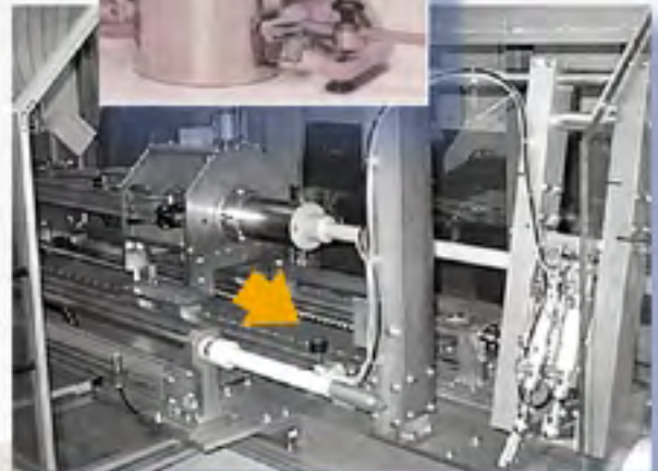
The reel machine for synthetic skins was developed according to the state of art. Fast and easy-running aluminium roller guides are used for the central horizontal movement. The large-dimensioned running rollers which rest on needle bearings and sustain loads from any direction.
