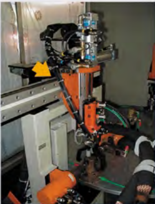
Aluminium roller guide in a welding machine. High accuracy and low weight for perfect welding.
