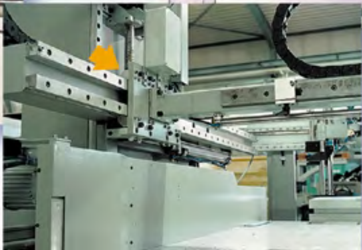
Handling device for paper stacks. The aluminium roller guides move jigs and stops reliably in permanent operation. (Photo Solms)
