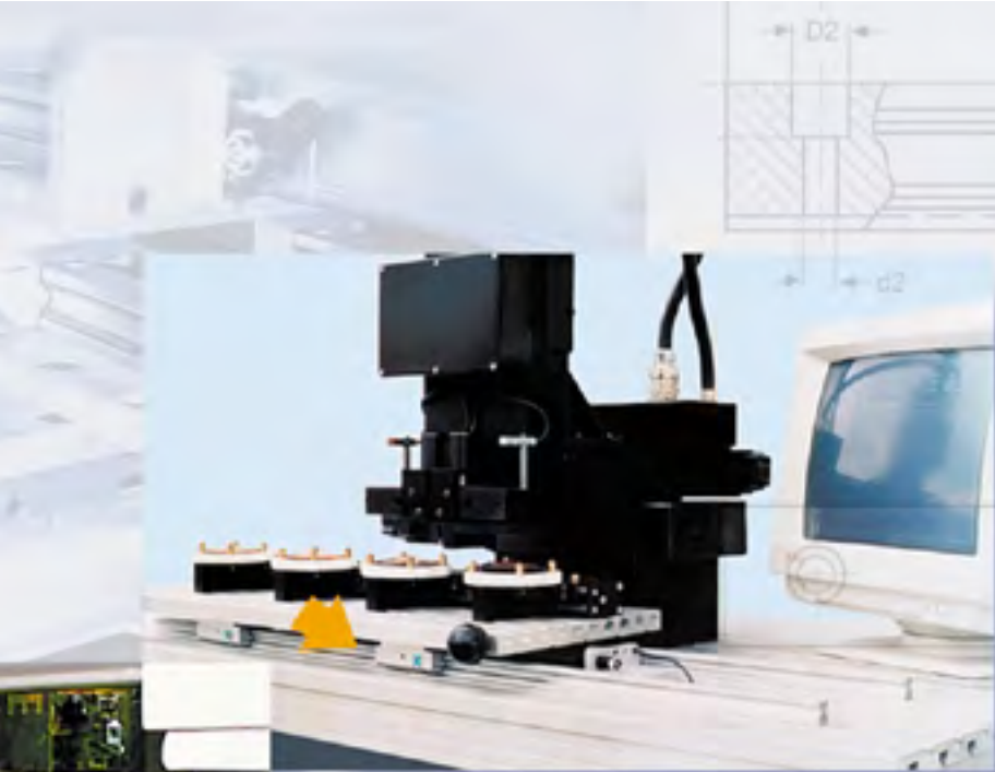
Aluminium roller guide in a glasses engraving machine. Work piece carrier and the motorized coordinate tables are equipped with roller guides. The very good running behaviour and precision of the installation allows extremely fine engraving. (Photo Kasch)
