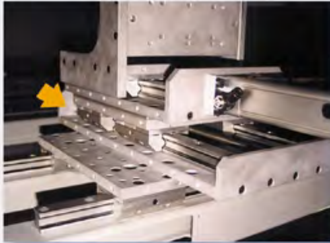
Multiaxis positioning unit for a welding machine. Tools and the material can be moved individually by aluminium roller guides.
