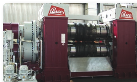
DESCH planetary gearbox, Denox P250-2-25-AHM type with attached torque motors for driving the top and bottom roller of a thermoforming rolling system
