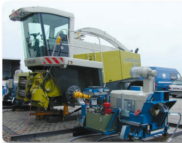
Test rig for drive lines of harvesters
