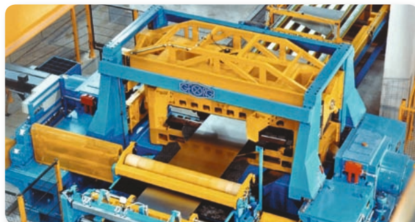
DESCH planetary gearbox in an eccentric shears
